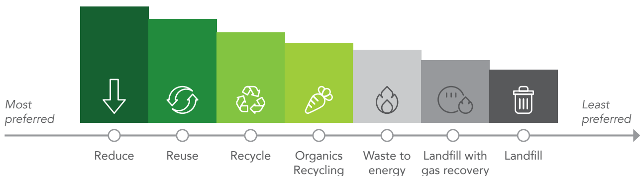
The solid waste management hierarchy ranks waste management methods from most to least preferred.
